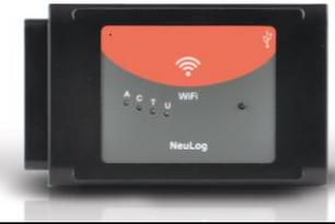
The next time the WiFi module is turned on it will again attempt to enter client mode by connecting to the same wireless connection. If the connection fails; the WiFi module will restart back in access point mode.
