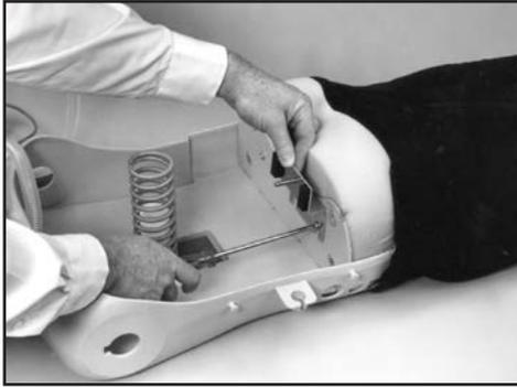
Once the bracket is in place with the single threaded screw and foam pads pointing towards the inner chest cavity, attach the load box to the screw sticking out and tighten until secure.
