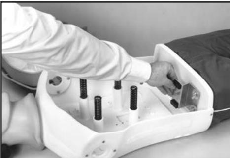
The bracket should be secured so that the foam pads and single screw stick out toward the chest cavity.
